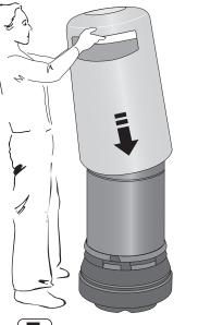
Lift bin body over liner and drop onto plinth to lock. Turn bin body to align apertures.
